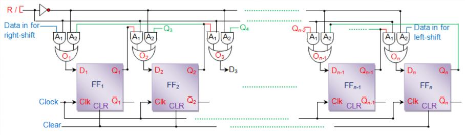
Figure 1 *n*-bit Bidirectional Shift Register
