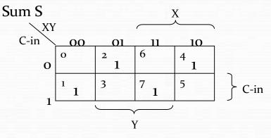
S = X'Y'(C-in) + XY'(C-in)' + XY'(C-in)' + XY(C-in) $S = X \oplus Y \oplus (C-in)$
